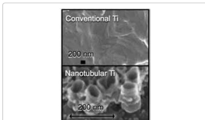
**Figure 1:** Conventional Ti implants (top) can be modified through an anodization process to create nanotubular Ti (bottom) which can improve cell responses, decrease inflammation, and decrease bacteria functions [15].
