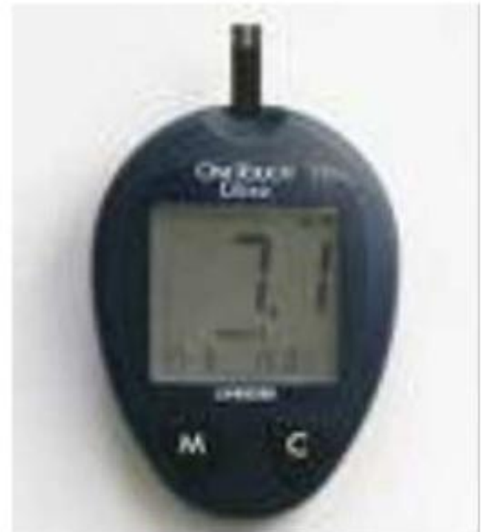
Glucometer- for measurement of glucose in blood.
