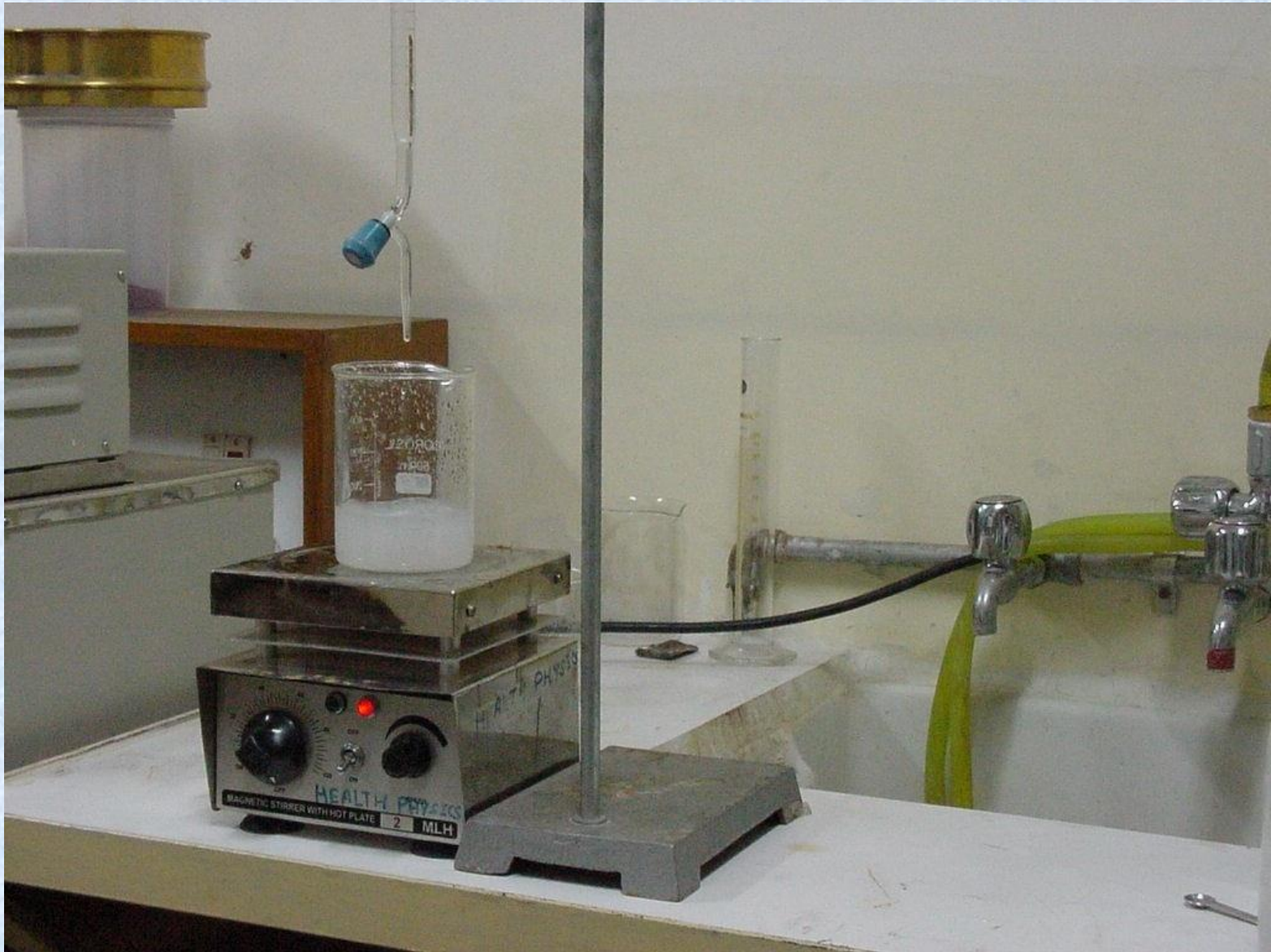
Set-up for preparing samples by Co-precipitation method
