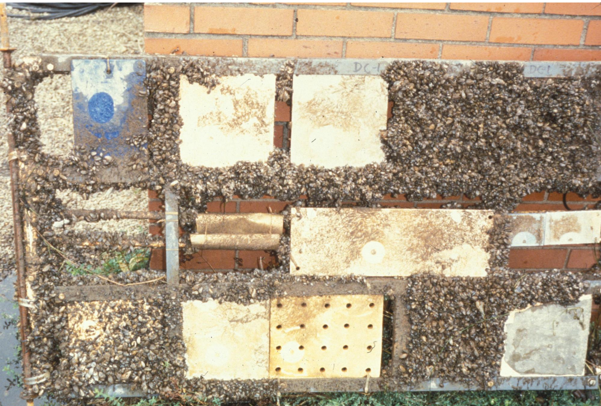
Test panels at Dunkirk, NY (zebra mussel fouling)
