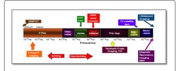
**Figure 6:** Frequency spectrum of electromagnetic radiation imaging technologies [15].
