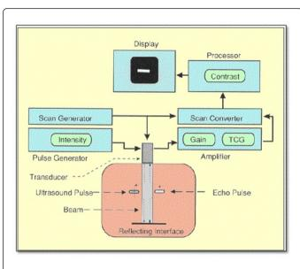
**Figure 4:** The principal functional components of an ultrasound imaging system [10].
