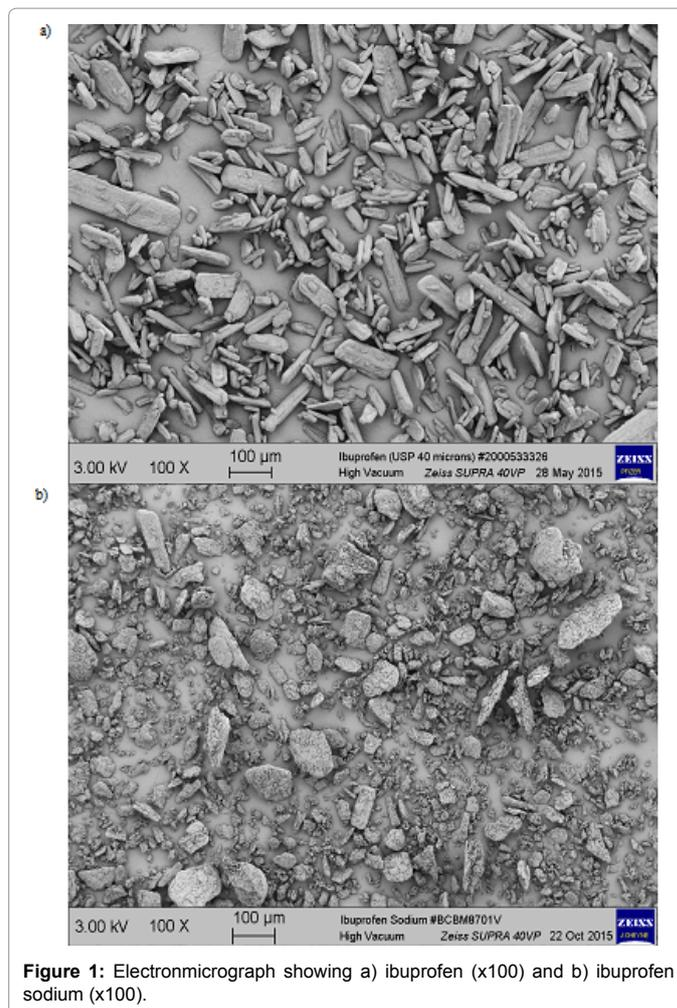
Figure 1: Electronmicrograph showing a) ibuprofen (x100) and b) ibuprofen sodium (x100).
