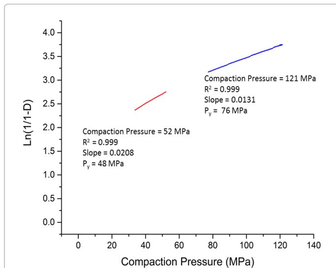
Figure 5: Derived yield pressure from Heckel plot at 52 MPa and 121 MPa.
