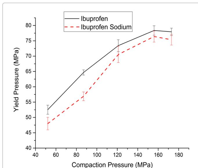
Figure 6: Effect of compaction pressure on yield for ibuprofen and ibuprofen sodium.
