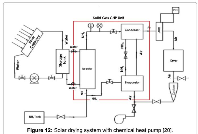
Figure 12: Solar drying system with chemical heat pump [20].
