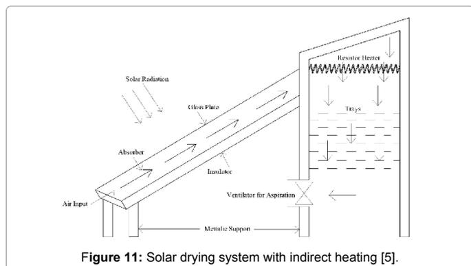
Figure 11: Solar drying system with indirect heating [5].
