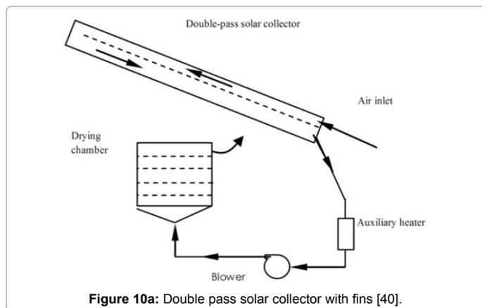
Figure 10a: Double pass solar collector with fins [40].
