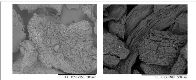
Figure 4: Scanning electron micrographs of GT (left) and PM (right) showing the heterogeneity of their surfaces.
