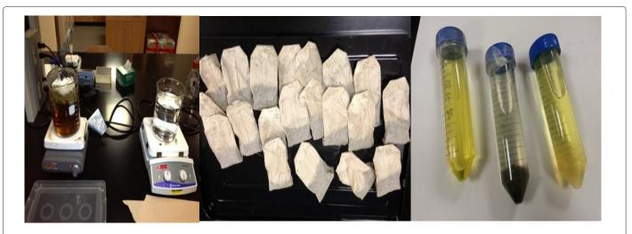
Figure 2: Preparation and adsorption experiments of the tea bag waste on the adsorption of dyes. (Left) Continuous boiling of tea bags; (Center) Tea bags of GT after boiling and drying; (Right) Adsorption of BY57 in batch experiments, showing control solution and with GT in the middle.
