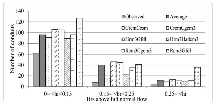
Figure 7: Number of conduits above full normal flow for 5 year return period storm.
