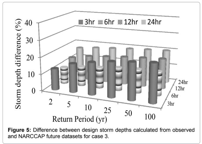
Figure 5: Difference between design storm depths calculated from observed and NARCCAP future datasets for case 3.
