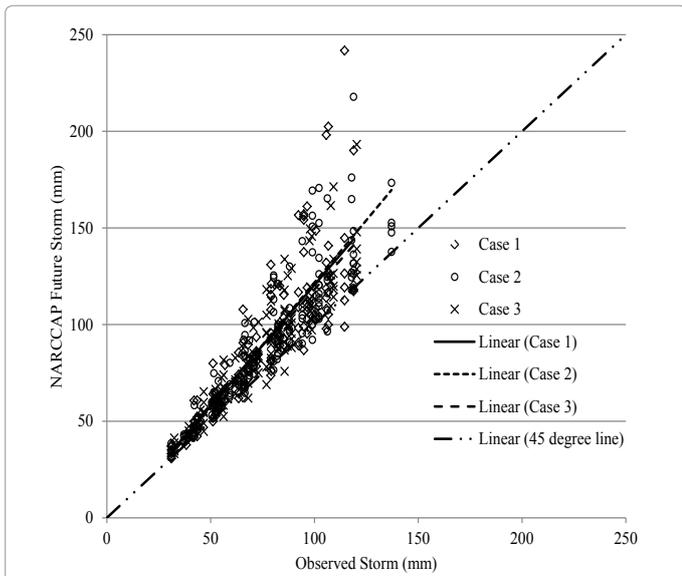
Figure 2: Scatterplot of design storm depths calculated from observed data and NARCCAP future datasets.
