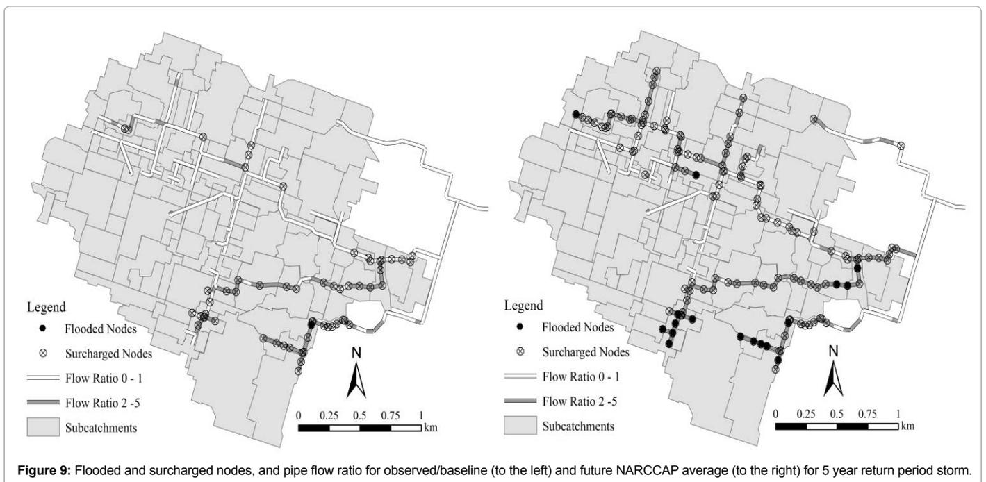
Figure 9: Flooded and surcharged nodes, and pipe flow ratio for observed/baseline (to the left) and future NARCCAP average (to the right) for 5 year return period storm.
