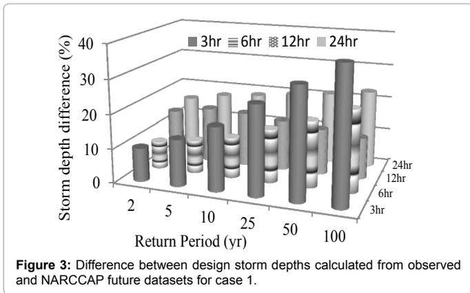
Figure 3: Difference between design storm depths calculated from observed and NARCCAP future datasets for case 1.
