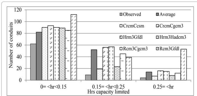
Figure 8: Number of conduits for capacity limited for 5 year return period storm.
