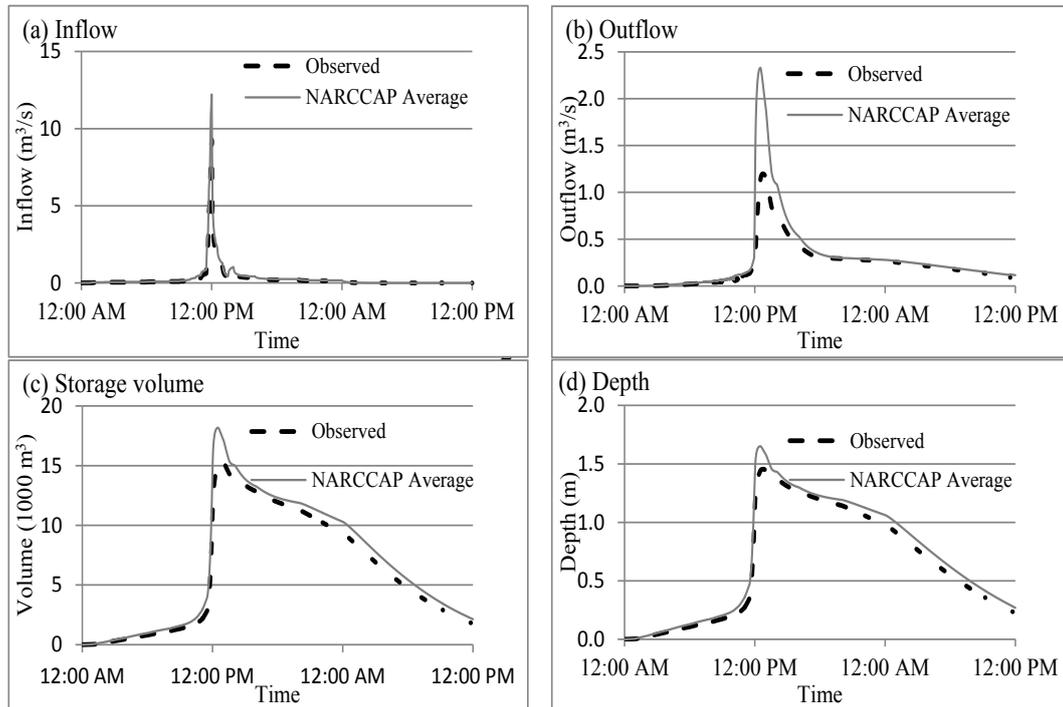
Figure 6: Plots showing time series of inflow, outflow, storage volume and depth from 25 year return period storm for detention pond 1 (observed/baseline values obtained using storm depths calculated from observed data).
