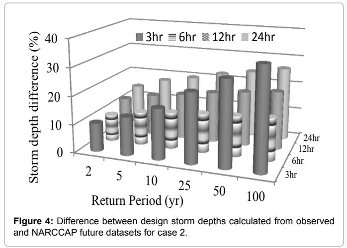
Figure 4: Difference between design storm depths calculated from observed and NARCCAP future datasets for case 2.
