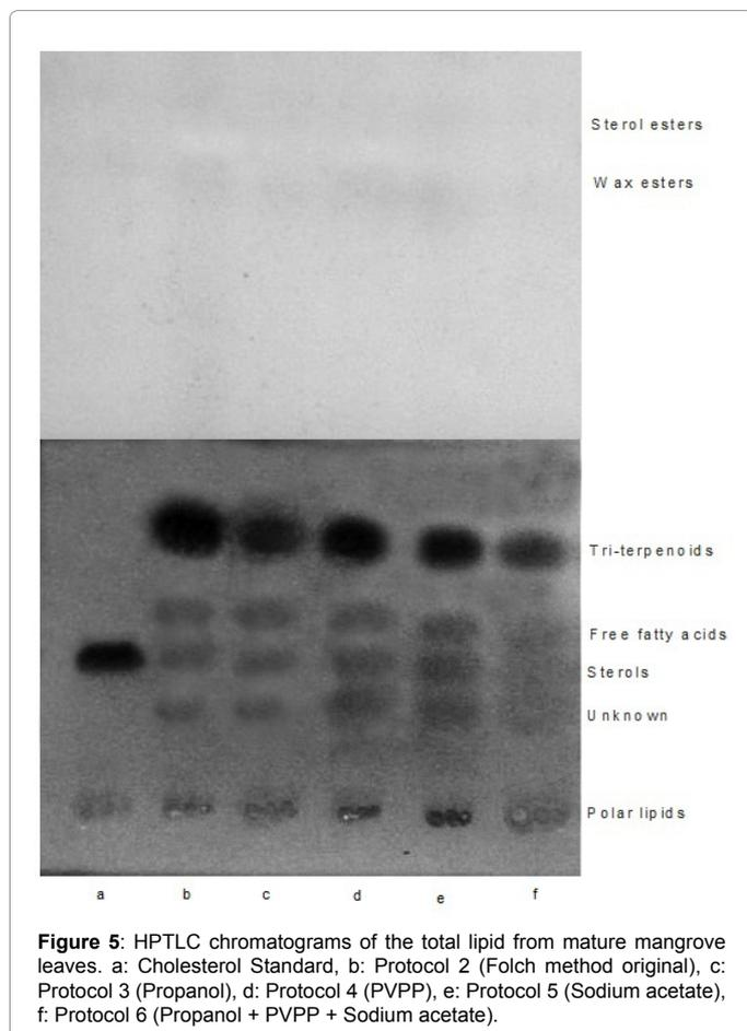
**Figure 5:** HPTLC chromatograms of the total lipid from mature mangrove leaves. a: Cholesterol Standard, b: Protocol 2 (Folch method original), c: Protocol 3 (Propanol), d: Protocol 4 (PVPP), e: Protocol 5 (Sodium acetate), f: Protocol 6 (Propanol + PVPP + Sodium acetate).
