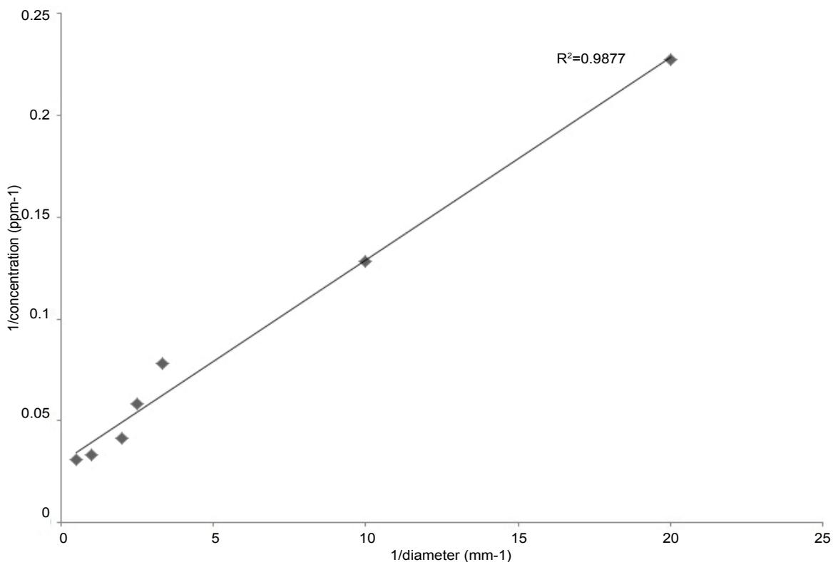
**Figure 7b:** A plot of 1/concentration (ppm<sup>-1</sup>) versus 1/diameter (mm<sup>-1</sup>) yields a linear relationship with an R<sup>2</sup> value of 0.987 indicates a reliance on surface site adsorption for 4NP deposition in snow.
