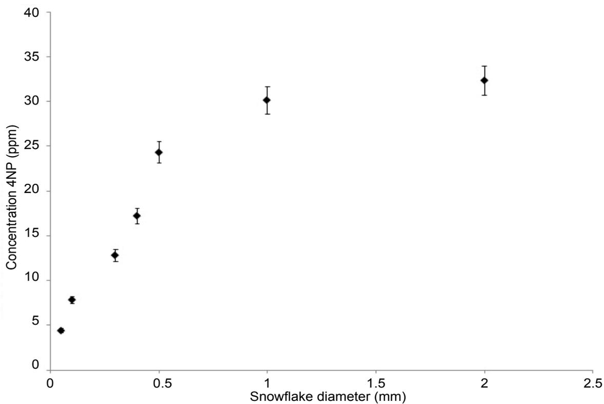
**Figure 7a:** The total concentration of 4NP deposited on snow pack with particles of variable diameter. 4NP was introduced by nebulizer at a rate of 1 m/s.
