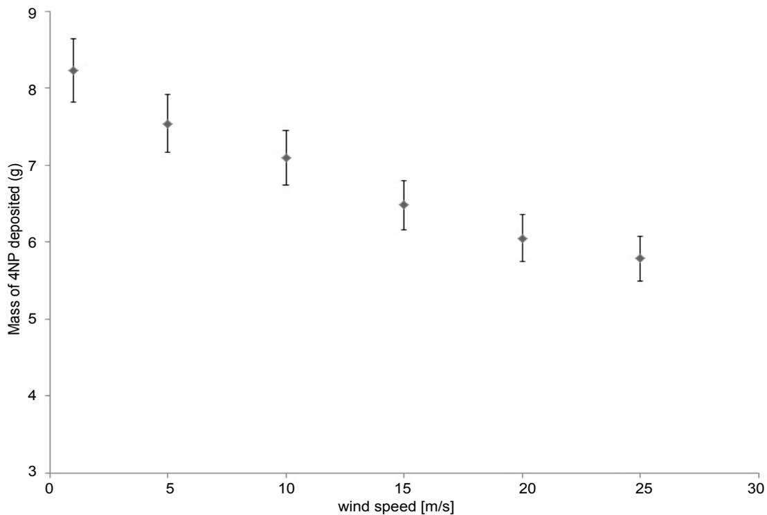
**Figure 8:** Snow chamber results of increasing wind speeds on 4NP aerosol deposition when snowflake size is held constant at 0.5 mm.
