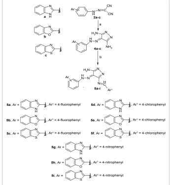
**Scheme 2:** Reagent and conditions: a) hydrazine hydrate 99%, reflux, 6 h; b) substituted aromatic aldehydes, DMF, glacial acetic acid, reflux, 12 h.
