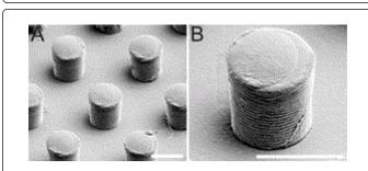
Figure 2: Low (A) and (B) high–magnification SEM images of 3D micropillared surface. 10  $\mu$ m bars.
