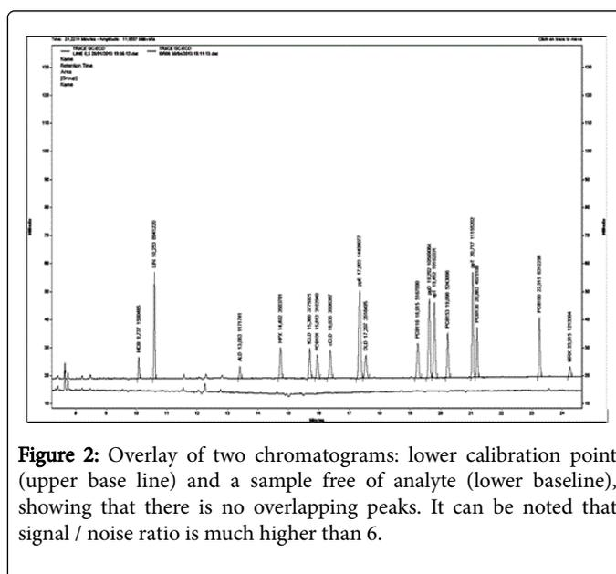
**Figure 2:** Overlay of two chromatograms: lower calibration point (upper base line) and a sample free of analyte (lower baseline), showing that there is no overlapping peaks. It can be noted that signal / noise ratio is much higher than 6.
