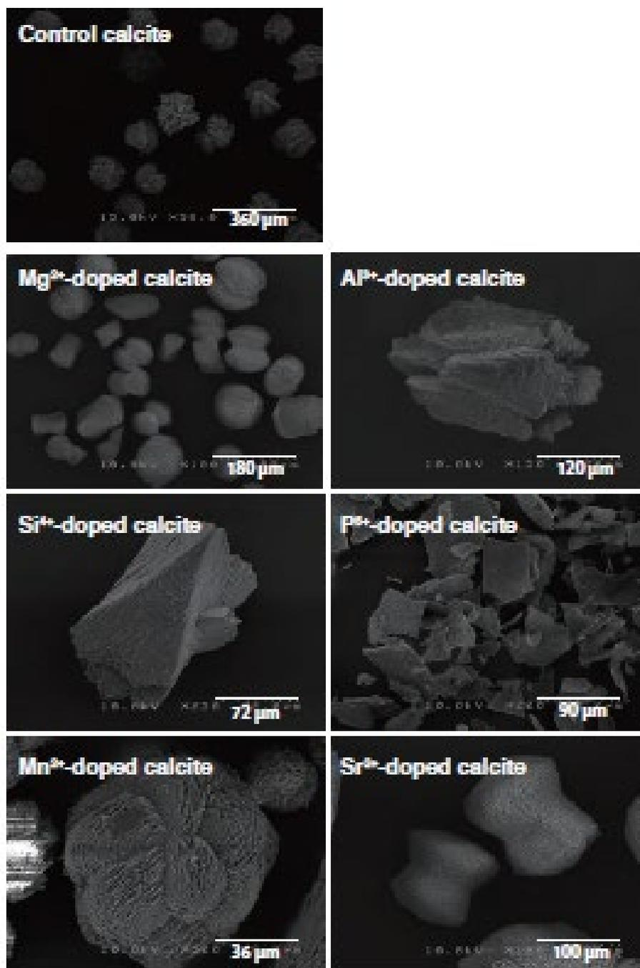
**Figure 2:** Scanning electron microscopy observations of calcite crystals synthesized within parent colonies. Calcite-promoting hydrogel was doped with different metal ions, as indicated in the upper left of each photograph. Control calcite was synthesized using standard calcite-promoting hydrogel.
