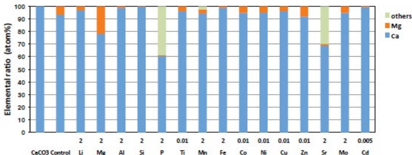
**Figure 1:** Elemental analysis of calcites synthesized on calcite-promoting hydrogels doped with different metal ions. The labels "CaCO<sub>3</sub>" and "control" indicate reagent-class pure calcium carbonate and calcite synthesized on standard calcite-promoting hydrogel, respectively. Numerals indicate the concentration (mM) at which each ion was doped in the respective standard calcite-promoting hydrogel.
