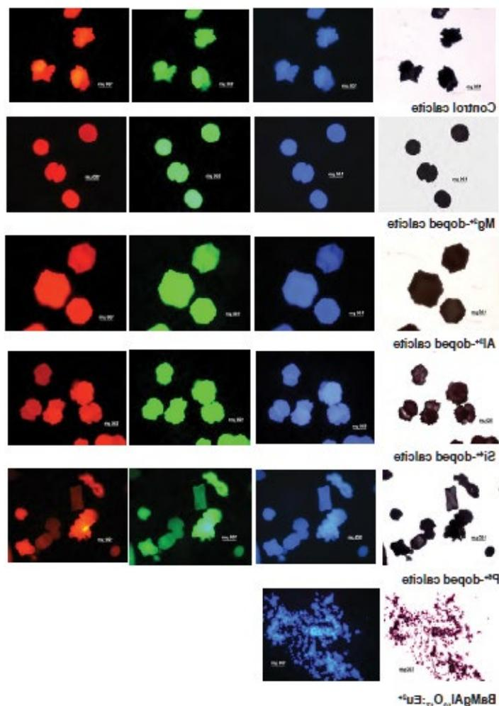
**Figure 4:** Fluorescence microscopy observations of calcite synthesized within parent colonies. Control calcite was synthesized using standard calcite-promoting hydrogel. Elemental ion-doped calcites were synthesized using calcite-promoting hydrogels doped with the indicated elemental ions at a concentration of 2 mM. Blue, green, and red emissions were observed at excitation wavelengths of 360-370 nm, 460-500 nm, and 530-560 nm, respectively.
