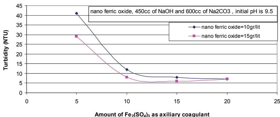
Figure 1: The effect of  $\text{Fe}_2(\text{SO}_4)_3$  on turbidity.
