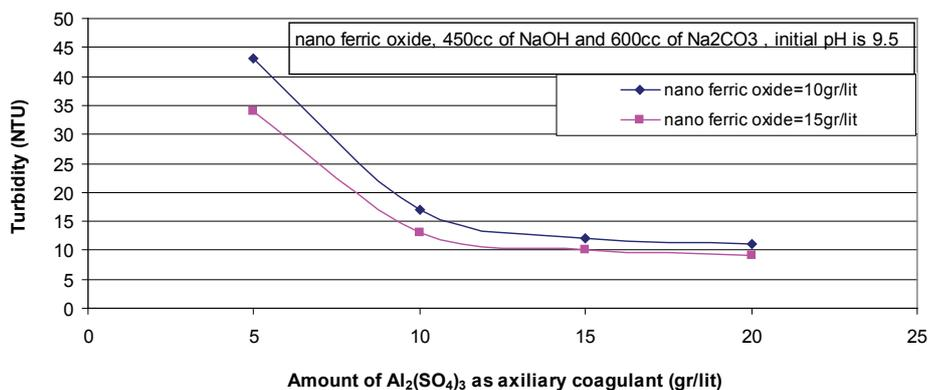
Figure 2: The effect of  $\text{Al}_2(\text{SO}_4)_3$  on turbidity.
