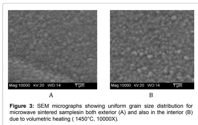
interspersed with the densely packed smaller grains (~ 0.3 μm) with the average grain size measured to be around 0.3 μm.
