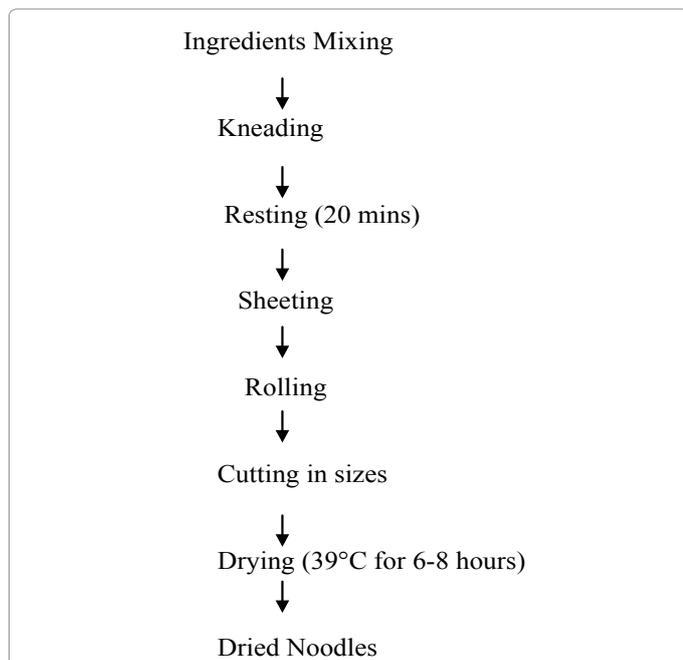
Figure 2: Production of trifoliate yam flour into noodles [14].
