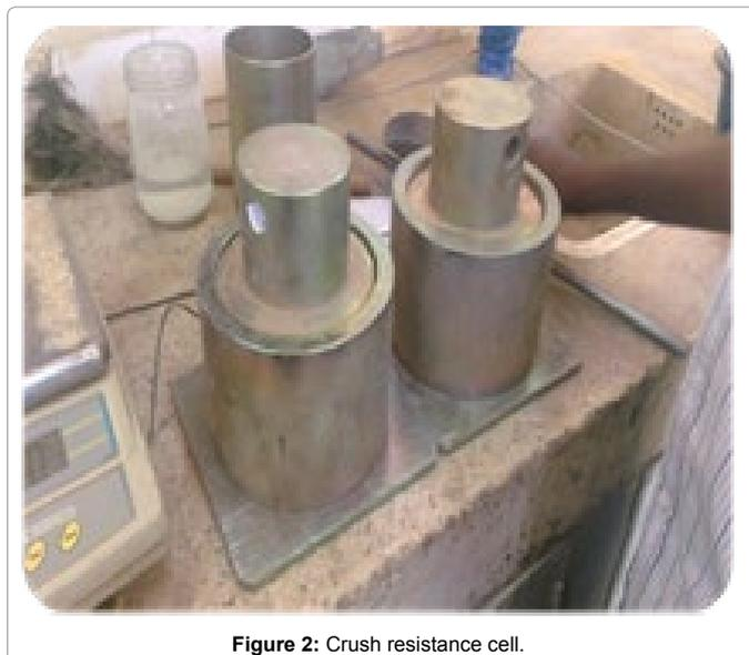
Figure 2: Crush resistance cell.
