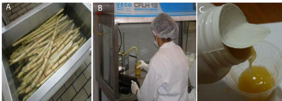
Figure 2: (a) Raw material, (b) Aseptic bottling and (c) Pasteurized sugarcane juice.
