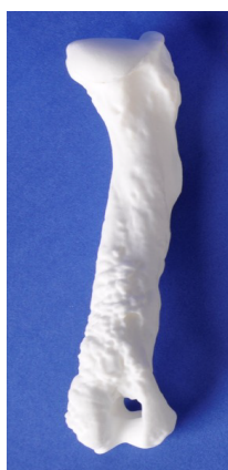
Figure 7: 3D Print (from CAD Model) of Abnormal Canine Humerus (Printing provided by Xometry Industrial 3D Printing & CNC Machining Services / photo courtesy of Mr. Thomas Martin, TU College of Veterinary Medicine Media Center).
