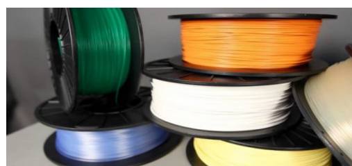
Figure 3: Poly-lactic Acid Filament, used in 3D printers, comes in a variety of colors (Photo courtesy of MakerBot.com).
