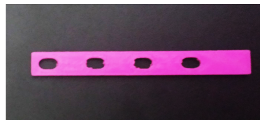
Figure 4: 3D printed sample of smaller version of orthopedic metal plate printed using Poly-lactic Acid (PLA), a plastic-type filament (Photo courtesy of Dr. D. Quinn-Gorham, TU College of Veterinary Medicine).
