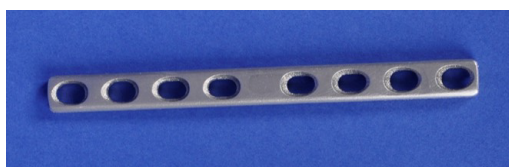
Figure 8: 3D Print (from CAD Model) of Orthopedic Metal Plate (Printing provided by Xometry Industrial 3D Printing & CNC Machining Services / Photo courtesy of Mr. Thomas Martin, TU College of Veterinary Medicine Media Center).
