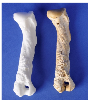
Figure 9: Comparison of 3D printed samples with originals. 3D printed bone (left side) and Original bone (right side) (Photos courtesy of Mr. Thomas Martin, TU College of Veterinary Medicine Media Center).
