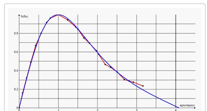
Figure 1.1: The proposed model for concrete compared with the experimental results.
