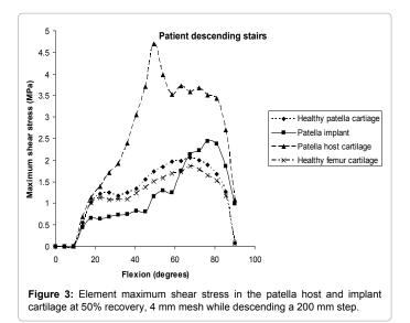
significant improvement. Shear stress reaches a peak of 2.5 MPa in the patella cartilage implant at 80° of flexion and 4.75 MPa in the host cartilage at 50° of flexion. The remaining pressure curves for the ACI at 50% recovery are lower than pressure values for healthy cartilage, which are to be expected when the Young's modulus of the cartilage has not yet developed to its full value.
