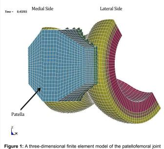
Figure 1: A three-dimensional finite element model of the patellofemoral joint at  $45^{\circ}$  flexion.
