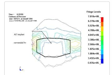
Figure 7: FEA plot of pressure contours (Pa) in the patella cartilage of patient A at 97.5% recovery of implant properties, 54° flexion and contact force of 2150N.
