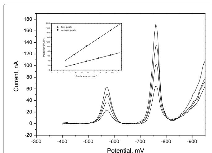
**Figure 4:** Voltammograms obtained for surface area of Hg (Ag) FE: 3.7, 5.7, 7.7 and 9.7 mm<sup>2</sup> for  $5 \cdot 10^{-7}$  M of isoniazid in 0.1 M CH<sub>3</sub>COOH. Instrumental parameters:  $\Delta E=30$  mV,  $E_s=4$  mV,  $t_w, t_p=10$  ms. Stirring rate, 500 rpm.
