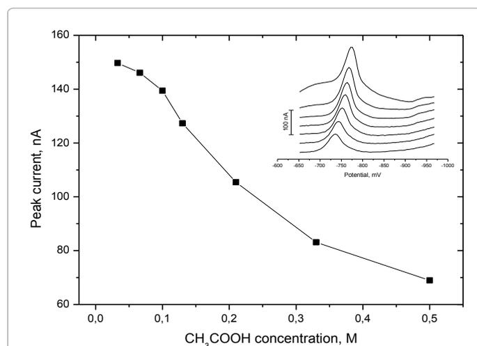
**Figure 3:** Effect of acetic acid concentration on peak current in short potential range, isoniazid concentration  $5 \cdot 10^{-7}$  M. Instrumental parameters:  $\Delta E=30$  mV,  $E_s=4$  mV,  $t_w, t_p=10$  ms. Stirring rate, 500 rpm.
