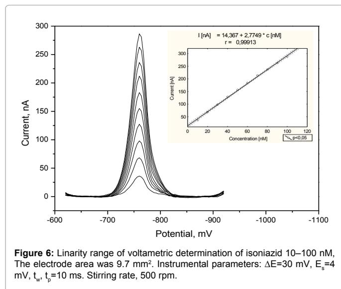
**Figure 6:** Linearity range of voltammetric determination of isoniazid 10–100 nM, The electrode area was 9.7 mm<sup>2</sup>. Instrumental parameters: ΔE=30 mV, E<sub>s</sub>=4 mV, t<sub>w</sub>, t<sub>p</sub>=10 ms. Stirring rate, 500 rpm.
