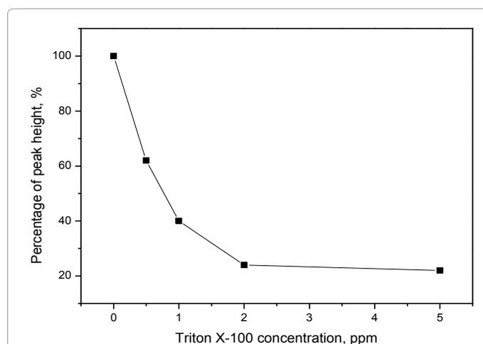
**Figure 5:** Influence of Triton X-100 addition in range 0.5 – 5 mgL<sup>-1</sup>, isoniazid concentration  $5 \cdot 10^{-7}$  M. Instrumental parameters:  $\Delta E=30$  mV,  $E_s=4$  mV,  $t_w, t_p=10$  ms. Stirring rate, 500 rpm.
