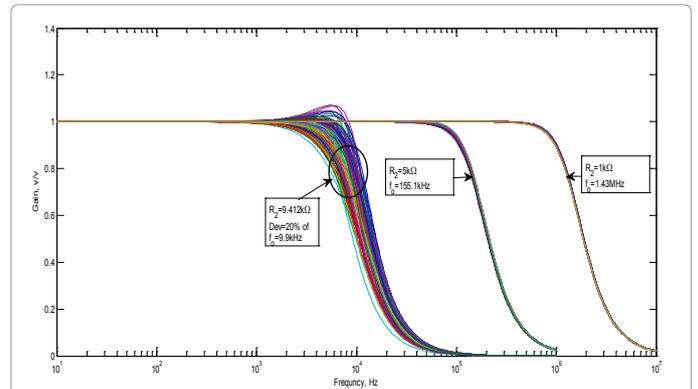
Figure 4: 2<sup>nd</sup> order LPF frequency responses for three different cases:  $R_2 = 9.4$ k $\Omega$  (downscaling),  $R_2 = 5$ k $\Omega$ ,  $R_2 = 1$ k $\Omega$  (up scaling).
