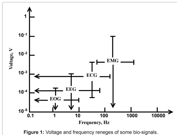
Figure 1: Voltage and frequency ranges of some bio-signals.
