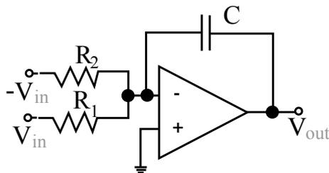
Figure 2: The integrator used for the frequency scaling approach.
