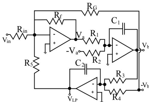
Figure 3: 2<sup>nd</sup> order Low Pass Filter applying difference approach topology.
