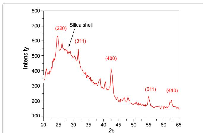
**Figure 3:** XRD profile of the core-shell structured MNPs; the small inset is the magnetization of IONPs as a function of temperature in the applied field of 50 Oe at a temperature range of 5 to 300 K using field 15 cooling (FC) and Zero-Field Cooling (ZFC) procedures.
