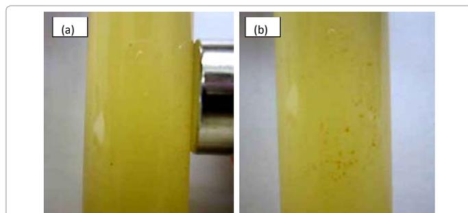
**Figure 7:** (a) Diluted *S. aureus* under external magnetic field (0.2 T). (b) Magnetic capture of diluted *S. aureus* in 1 min.
