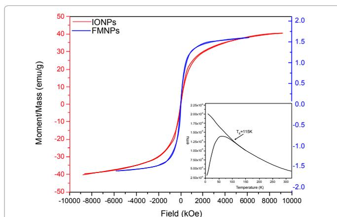
**Figure 4:** Hysteresis loops of iron oxide nanoparticles and the core-shell structure.
