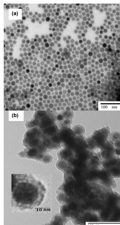
Figure 2: TEM micrographs of (a) iron oxide nanoparticles, and (b) core-shell structured MNPs
