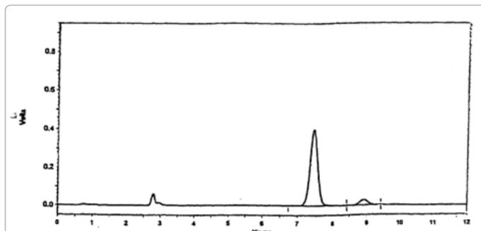
Figure 1: HPLC chromatogram showing human plasma containing 150 ng/ml ciprofloxacin at retention time 9 min and internal standard levofloxacin peak at 7 min.
