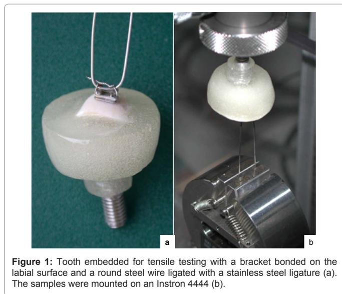
**Figure 1:** Tooth embedded for tensile testing with a bracket bonded on the labial surface and a round steel wire ligated with a stainless steel ligature (a). The samples were mounted on an Instron 4444 (b).
