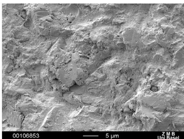
**Figure 3:** SEM image of an enamel surface after air abrasion with 50 μm Al<sub>2</sub>O<sub>3</sub> particles.
