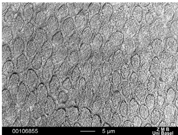
**Figure 2:** SEM image of an enamel surface etched for 15 s with 37% H<sub>3</sub>PO<sub>4</sub>.
