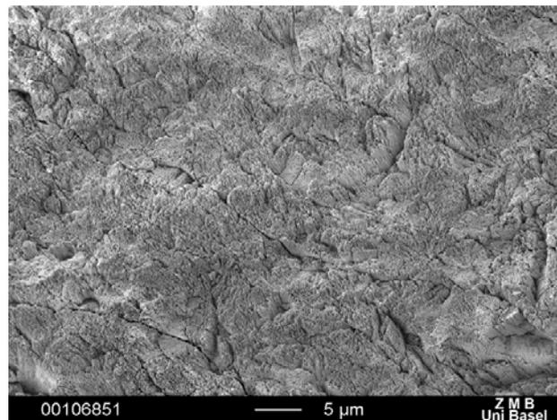
**Figure 4:** SEM image of an enamel surface after air abrasion with 50 μm Al<sub>2</sub>O<sub>3</sub> particles and additional etching with 37% H<sub>3</sub>PO<sub>4</sub> for 15 s.
