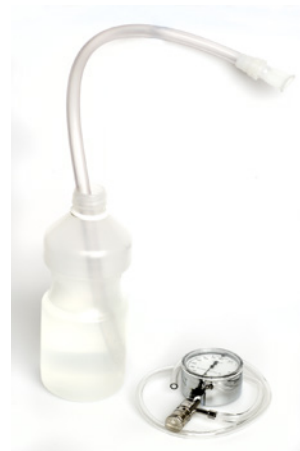
Figure 1: The Blow bottle system and a pressure manometer. The pressure is adjusted by varying the quantity of water in the bottle.
