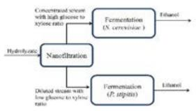
Fig. : Proposed strategy for processing of hydrolyzate from lignocellulosic biomass via nanofiltration
