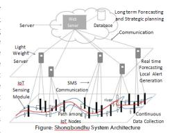
the river banks and once the water level rises above the danger level, alert messages are generated and disseminated to predefined phones and systems. The system has been tested in laboratories as well as along the river banks in Dhaka, Bangladesh. The current system shows more than 99% of accuracy in real time water level detection and alert generation.
