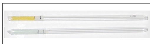
Figure-1: Cathinone detector tube. Approximately 100 \mu L of a test solution is sucked into the detector tube. Upper one is positive control. Orange color appeared in the presence of cathinones.
