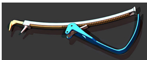
Figure 2: Visualization of the designed forceps for mandible fracture reduction.
