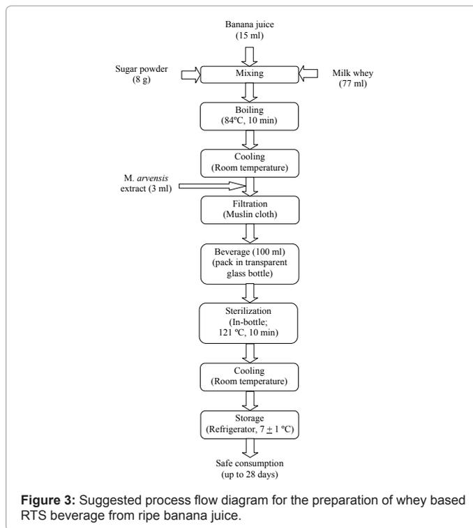
**Figure 3:** Suggested process flow diagram for the preparation of whey based RTS beverage from ripe banana juice.
