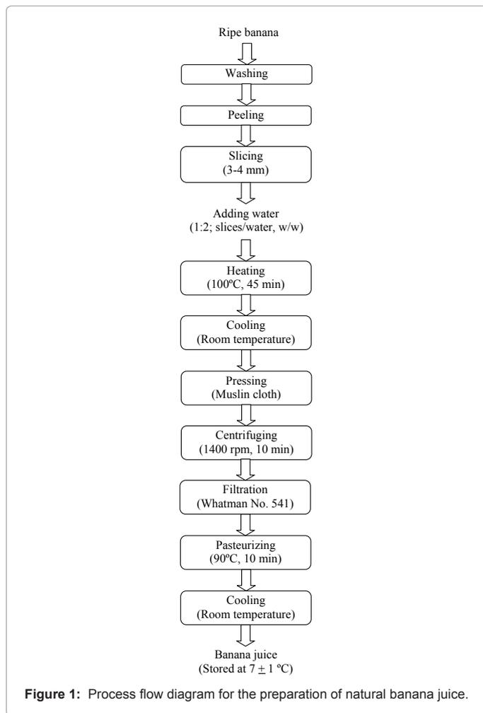
slices of 3-4 mm. The banana slices along with RO purified water in the ratio of 1:2 (banana slice : water, w/w) were heated at 100°C for 45 minutes followed by the cooling, pressing, centrifuging (at 1400 rpm for 10 min), filtration, pasteurization (at 90°C for 10 min) and again cooling at room temperature. The prepared banana juice was stored at 7 ± 1°C temperature in the refrigerator for further use in the RTS beverage preparation.
