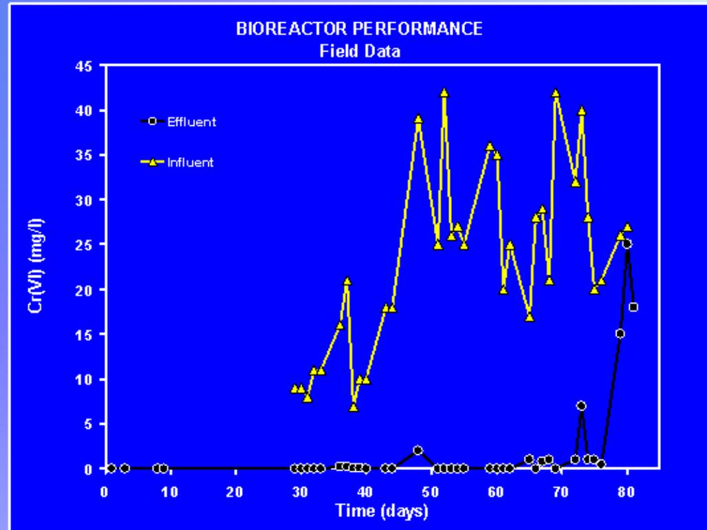
Our technology was incorporated into a 30,000 liter industrial bioreactor to remove Cr(VI) from waste leachate at a chromium steel factory in Sweden. Indigenous Cr(VI) reducing bacteria dominated the bioprocess that was fed acetate waste from a neighboring industry. The resulting Cr(III) precipitated inside the bioreactor as a hydroxide.
