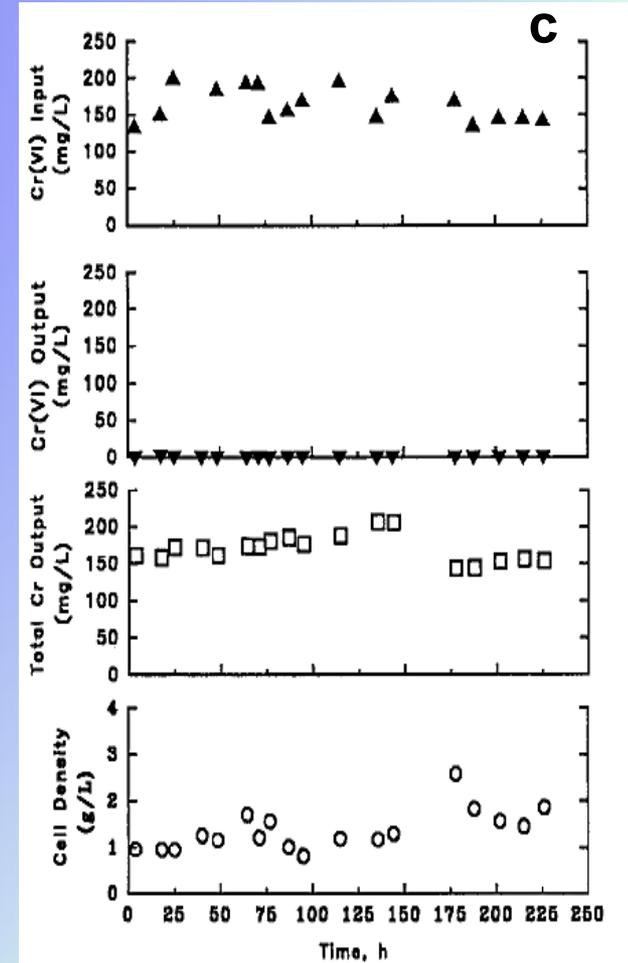
Incorporating a mixed culture of Cr(VI) reducing bacterial biofilm into a bioreactor (a) demonstrated that a robust mixed culture could be isolated from the environment. The mixed culture biofilm grew well across a wide range of Cr(VI) concentrations (b) and reduced about 200 mg/l of Cr(VI) with a 48 hr. retention time (c).
