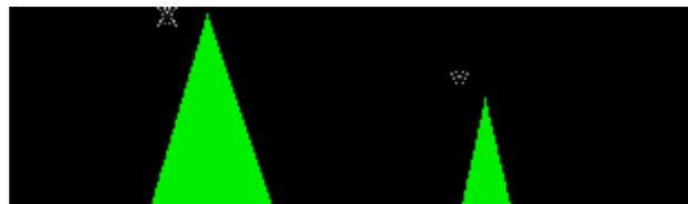
In the diagram, the area under the peak for Y is less than that for X. That may be because there is less Y than X, but it could equally well be because Y absorbs UV light at the wavelength you are using less than X does. There might be large quantities of Y present, but if it only absorbed weakly, it would only give a small peak.
