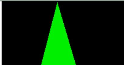
If the solution of X was less concentrated, the area under the peak would be less - although the retention time will still be the same. For example:
