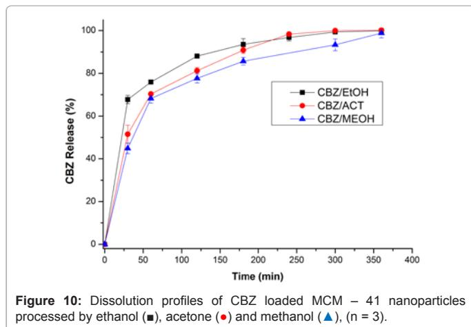
Figure 10: Dissolution profiles of CBZ loaded MCM – 41 nanoparticles processed by ethanol (■), acetone (●) and methanol (▲), (n = 3).
