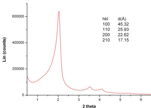
Figure 6: X – ray diffractogram of pure MCM-41 nanoparticles synthesized by the sol – gel process.
