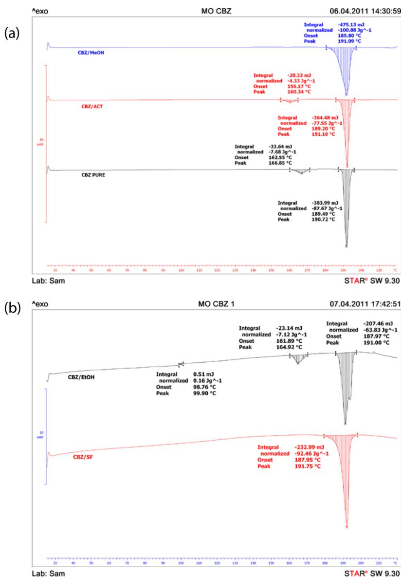
Figure 9: DSC thermograms of a) CBZ loaded MCM – 41 nanoparticles process by acetone, methanol – pure CBZ (bottom) and b) ethanol and control (processed only with CO<sub>2</sub>).
