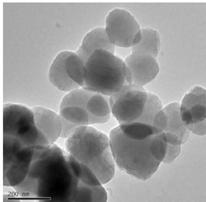
Figure 5: Transmission electron micrograph of MCM-41 nanoparticles.
