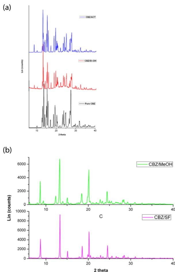
Figure 8: XRD patterns of a) CBZ loaded MCM – 41 nanoparticles process by acetone, ethanol – pure CBZ (bottom) and b) methanol and control (processed only with  $CO_2$ ).
