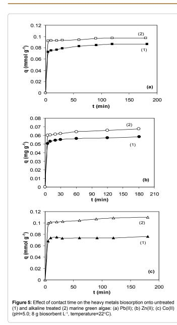
In comparison with the pseudo-first order kinetic model, the pseudo-second order kinetic model is based on the assumption that the rate controlling step in the biosorption mechanism is chemical interaction between metal ions and superficial functional groups of biosorbent. The mathematical expression of the pseudo-second order kinetic model can be written in linear form as [31,33]:
