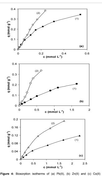
respectively, onto untreated (1) and alkaline treated (2) marine green algae (pH=5.0; 8 g biosorbent L<sup>-1</sup>, temperature=22°C; contact time=24 hours).
