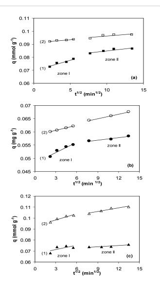
**Figure 6:** The plots of intra-particle diffusion model for the biosorption of (a) Pb(II), (b) Zn(II) and (c) Co(II) respectively, onto untreated (1) and alkaline treated (2) marine green algae.
