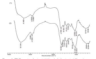
Figure 2: FT-IR spectra of untreated (1) and alkaline treated (2) marine green algae (*Ulva lactuca*).
