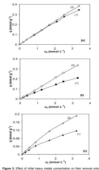
Figure 3: Effect of initial heavy metals concentration on their removal onto untreated (1) and alkaline treated (2) marine green algae: (a) Pb(II); (b) Zn(II); (c) Co(II) (pH=5.0; 8 g biosorbent L<sup>-1</sup>, temperature=22°C; contact time=24 hours).
