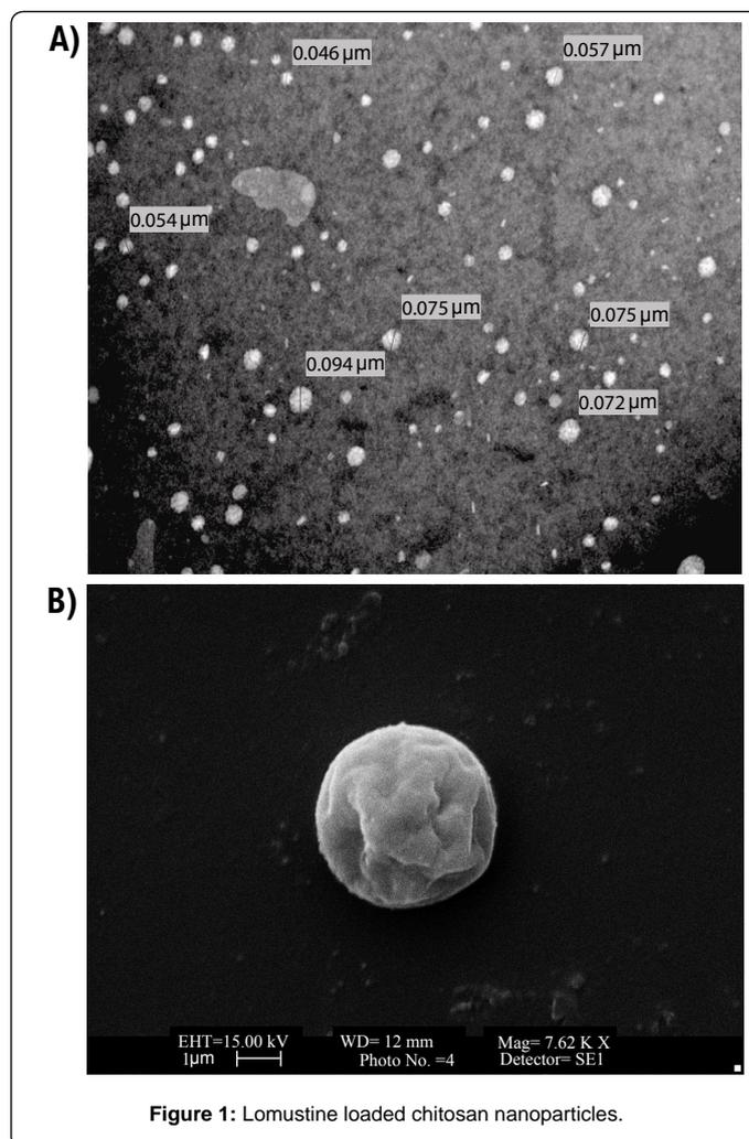
Figure 1: Lomustine loaded chitosan nanoparticles.
