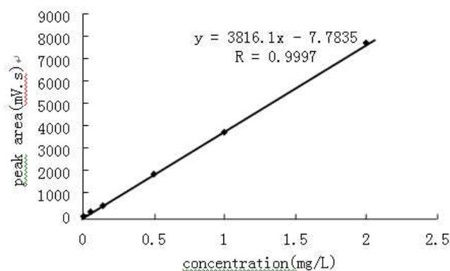
Figure 2: Calibration curve for prochloraz (concentration from 0-2.0 mg/L).
