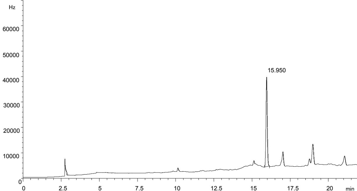
Figure 3: Chromatogram of 0.5mg/kg 2,4,6-trichloro-phenol.
