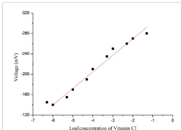
**Figure 2:** Calibration curve using enzyme immobilized ZnO-nanorods based biosensor electrode representing the electrochemical response (EMF) at different L-ascorbic acid concentrations  $1 \times 10^{-6}$  to  $5 \times 10^{-2} \text{ M}$  with Ag/AgCl reference electrode.
