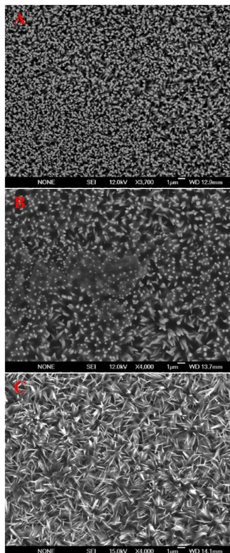
**Figure 1(a-c):** Typical field emission scanning electron microscopy (FESEM) images of ZnO nanorods grown on gold coated glass substrate using hydrothermal growth method. Figure (a) showing the ZnO-nanorods as grown (b) with immobilized ascorbate oxidase enzyme (c) and same used biosensor.
