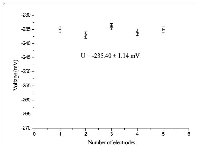
**Figure 3:** Calibration curve representing the biosensor to biosensor reproducibility in  $5 \times 10^{-5} \text{ M}$  ascorbic acid test solution.
