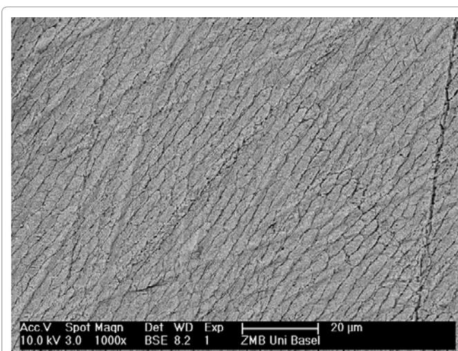
Figure 1: Typical surface after conventional etching with 37% phosphoric acid for 30s.
