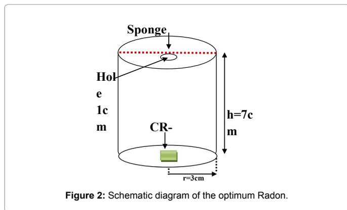
from the outside and that only radon gas, among other constituents, diffuses through it to the sensitive volume of the chamber. The design of the chamber ensures that the aerosol particles and radon decay products are deposited on the sponge from outside and only radon, among other gases, diffuses through it to the sensitive volume of the chamber. The calibration process for the dosimeter of this type and dimension was done by Ismail and Jaafar [7].
