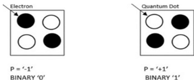
Figure 2: Figure showing two stable states of polarization in a basic QCA cell.
