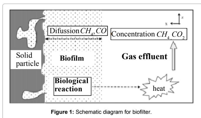
Figure 1: Schematic diagram for biofilter.
