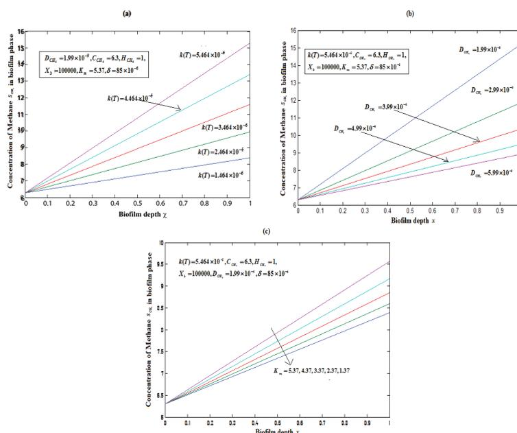
Figure 2: a-c. Concentrations of methane in biofilm phase versus coordinate of biofilm depth for different values of the parameters using Eqn.(12).
