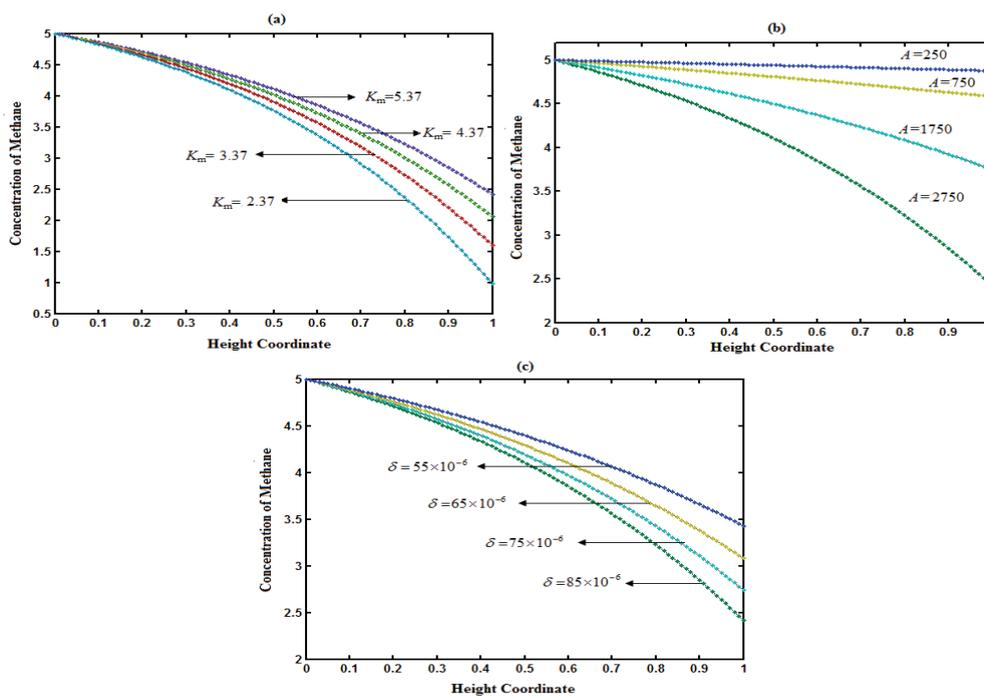
Figure 4: a-c. Concentrations of the Methane in gas phase methane versus coordinate of height for different values of the parameters using Eqn. (15).
