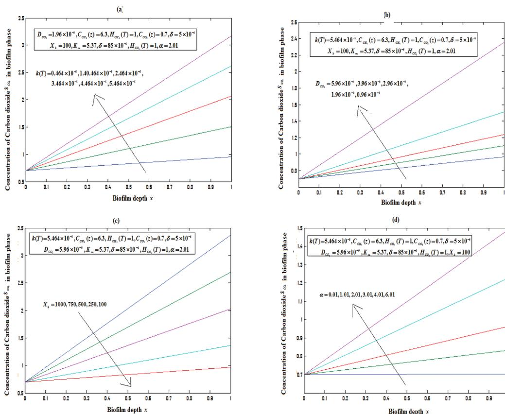
Figure 3: a-d. Concentrations of the Carbon dioxide in biofilm phase versus coordinate of biofilm depth for different values of the parameters using Eqn.(13).
