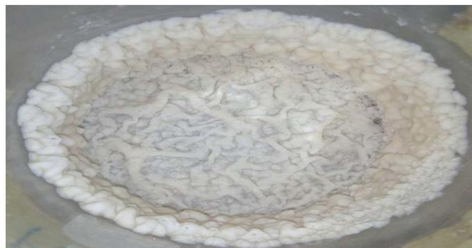
**Figure 5:** Plate 2: Chitosan hydrogel produced when chitosan was dissolved in 1% acetic acid and concentrated at 75°C.
