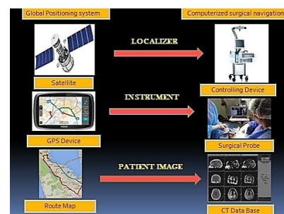
Figure 1: Hypothetical representation of surgical navigation surgery, emphasizing on its resemblance of each of its basic components with global positioning system, (1) The localizer (main controlling device for integration, replication and virtual reproduction of anatomical structures) works as a satellite. (2) A surgical probe which sends signals through infrared diodes or pointers and mimics the GPS system in the vehicle, as it emits track waves. (3) A computerized tomography database, for identification of abnormalities and confirming postoperative surgical results, is similar to the road map depicted in GPS system for route navigation.
