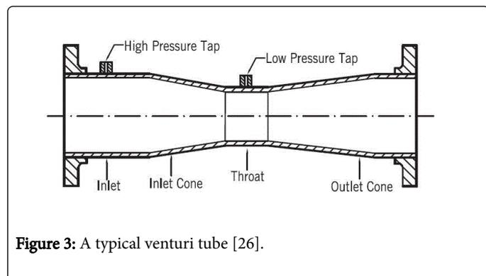
**Figure 3:** A typical venturi tube [26].
