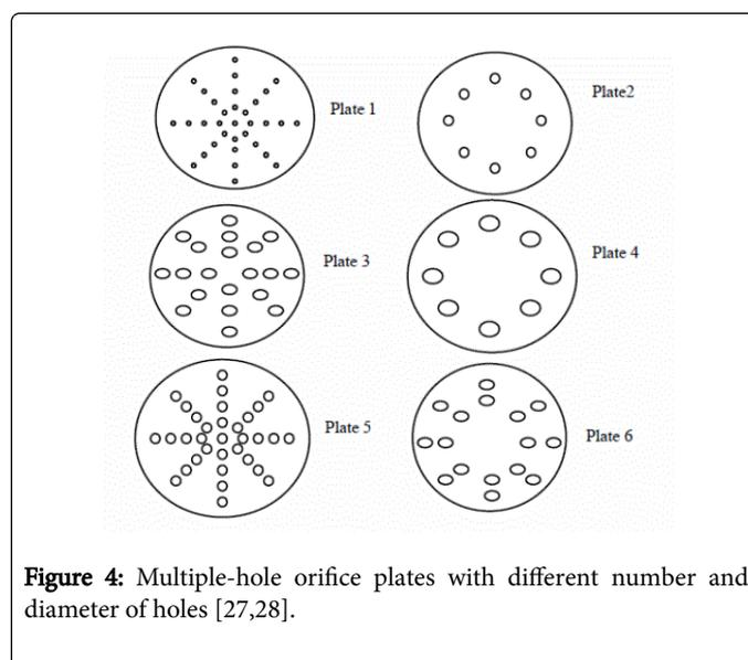
**Figure 4:** Multiple-hole orifice plates with different number and diameter of holes [27,28].
