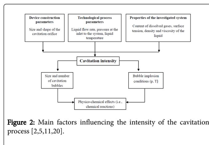
**Figure 2:** Main factors influencing the intensity of the cavitation process [2,5,11,20].
