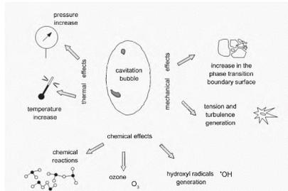
**Figure 1:** Physicochemical effects produced during the cavitation process [4].
