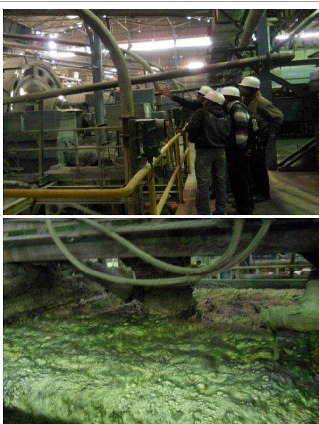
Figure 1: MCP concentrator plant (up), concentrated copper generation chamber by flotation method at MCP concentrator plant (down).
